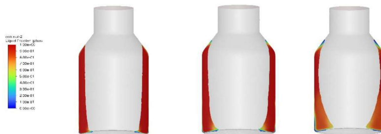
Figure 4: Liquid fraction of solution after 0.1 , 0.25, and 0.4 s from left to right respectively
